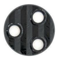
This electrodeposition process is recommended for creating a primer coat on the surfaces of elements made of iron, steel and other alloys. It offers excellent resistance to atmospheric corrosion and other forms of attack, and improves the adhesion of powder coatings. This type of coating has poor resistance to UV exposure, and is therefore not suitable for use in direct sunlight.
